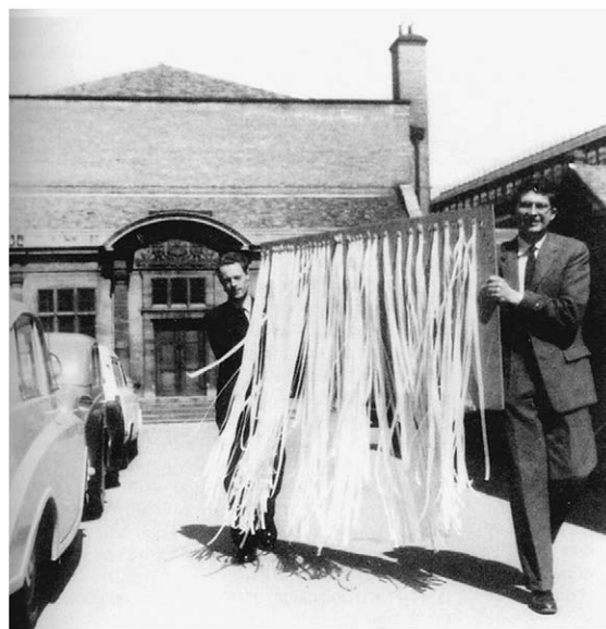
Fig. 3.7. Dick and Bror with the myoglobin sorting board. Each piece of punched tape represented a set of intensities from one line (constant h and k ) of reflections on one precession photograph. The same line of reflections might have been recorded on a number of photographs, thus permitting the determination of scale factors between photographs.
