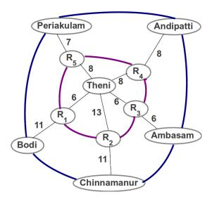
The black lines connect the remote locations (ex: Andipatti) to the hospital in Theni using relays; the black lines indicate wireless connections and the cost of using the wireless link
