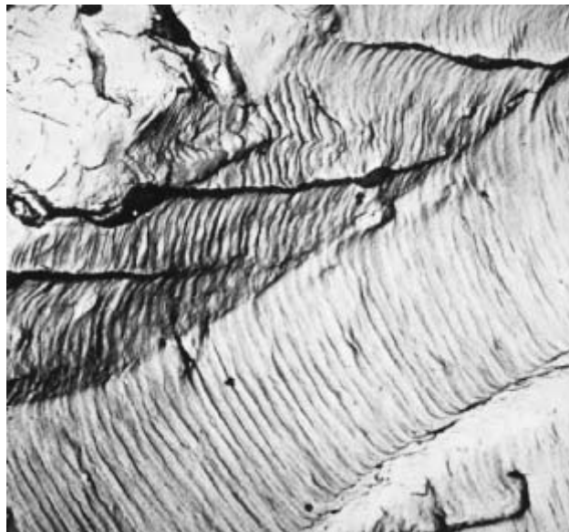
FIGURE 8.13W Transmission electron fractograph showing fatigue striations in aluminum. Magnification unknown. (From V. J. Colangelo and F. A. Heiser, Analysis of Metallurgical Failures , 2nd edition. Copyright © 1987 by John Wiley & Sons, New York. Reprinted by permission of John Wiley & Sons, Inc.)
