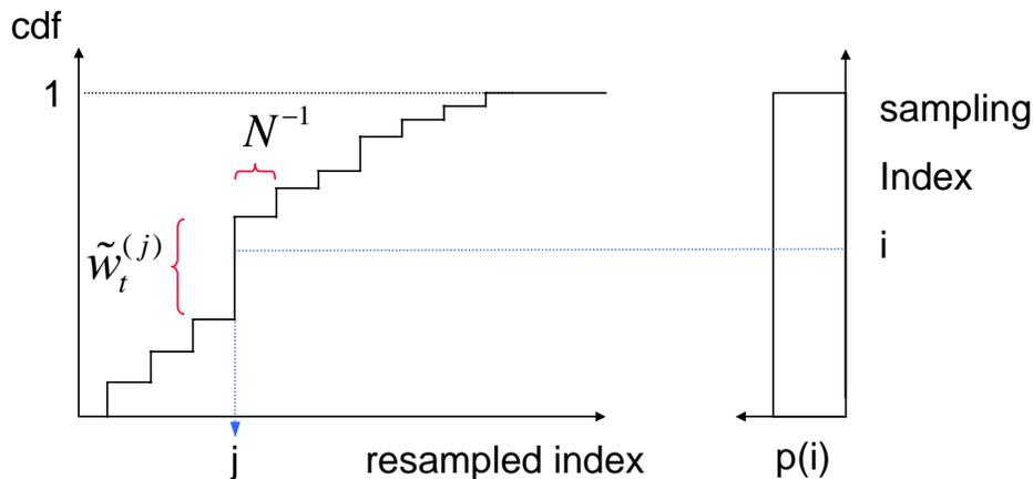
Figure 3: Resampling process, whereby a random measure  $\{\mathbf{x}_{1:t}^{(i)}, \tilde{w}_t^{(i)}\}$  is mapped into an equally weighted random measure  $\{\mathbf{x}_{1:t}^{(j)}, N^{-1}\}$ . The index  $i$  is drawn from a uniform distribution.
