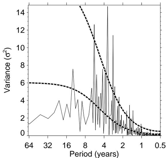
FIG. 3. Fourier power spectrum of Niño3 SST (solid), normalized by  $N/(2\sigma^2)$ . The lower dashed line is the mean red-noise spectrum from (16) assuming a lag-1 of  $\alpha = 0.72$ . The upper dashed line is the 95% confidence spectrum.
