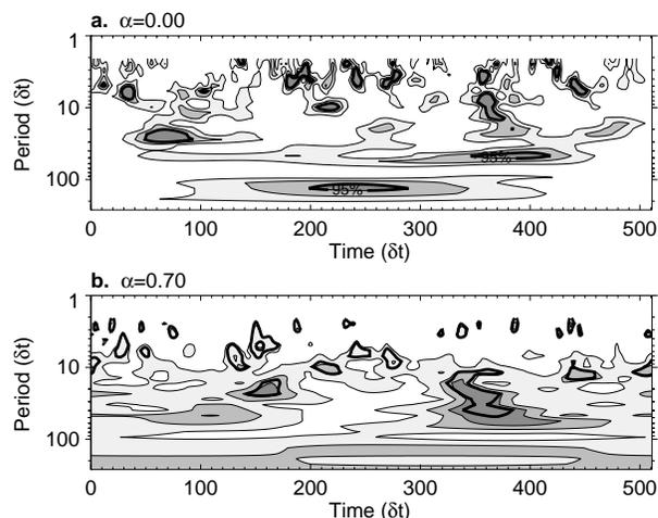
FIG. 4. (a) The local wavelet power spectrum for a Gaussian white noise process of 512 points, one of the 100 000 used for the Monte Carlo simulation. The power is normalized by  $1/\sigma^2$ , and contours are at 1, 2, and 3. The thick contour is the 95% confidence level for white noise. (b) Same as (a) but for a red-noise AR(1) process with lag-1 of 0.70. The contours are at 1, 5, and 10. The thick contour is the 95% confidence level for the corresponding red-noise spectrum.
