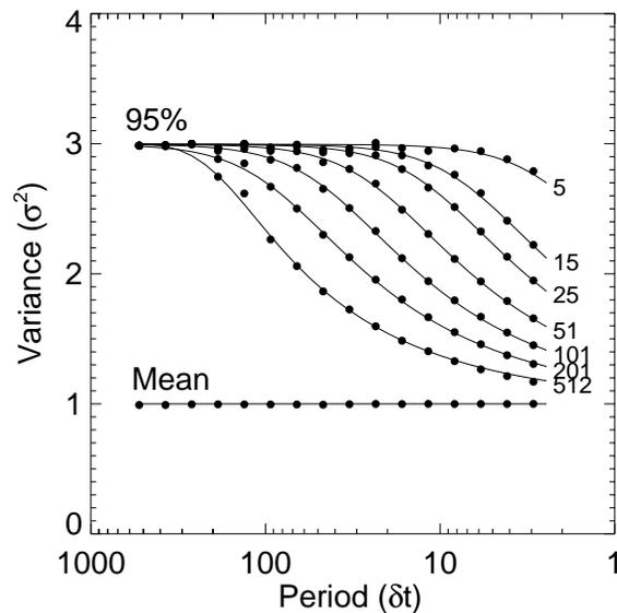
FIG. 7. Monte Carlo results for the time-averaged wavelet spectra (21) of white noise using the Morlet wavelet. The numbers to the right of each curve indicate  $n_a$ , the number of times that were averaged, while the black dots are the 95% level for the Monte Carlo runs. The top thin lines are the 95% confidence from (23). The lower thin line is the mean white-noise spectrum, while the black dots are the means of the Monte Carlo runs (all of the means are identical).
