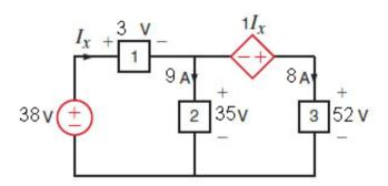
Let's calculate the power absorbed by elements where we know both voltage and current.
