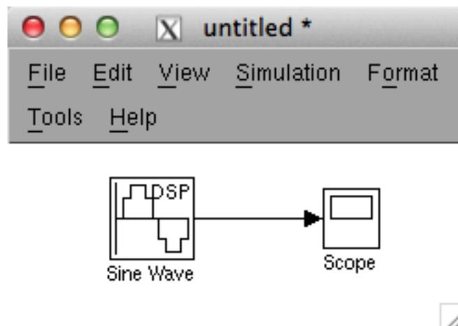
Figure 5. Completed System for Viewing Sine Wave
