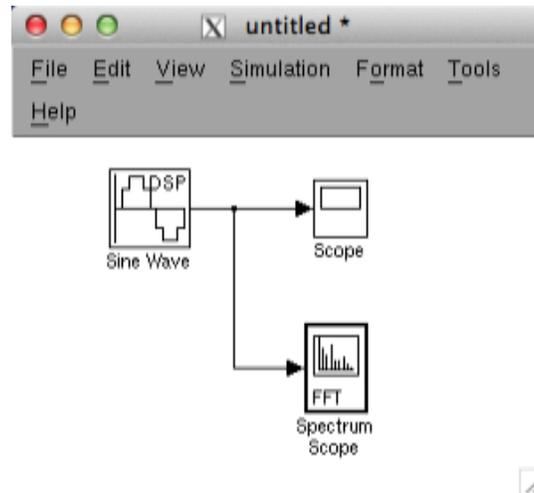
Figure 7. Power Spectral Density Sink
