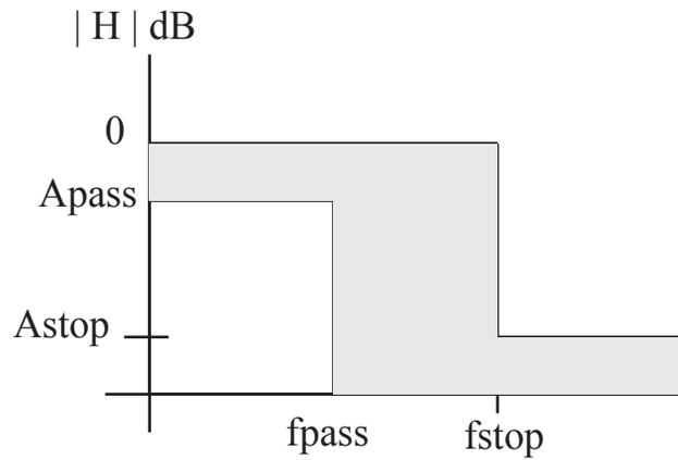
Figure 13. Frequency Response of Lowpass Filter
