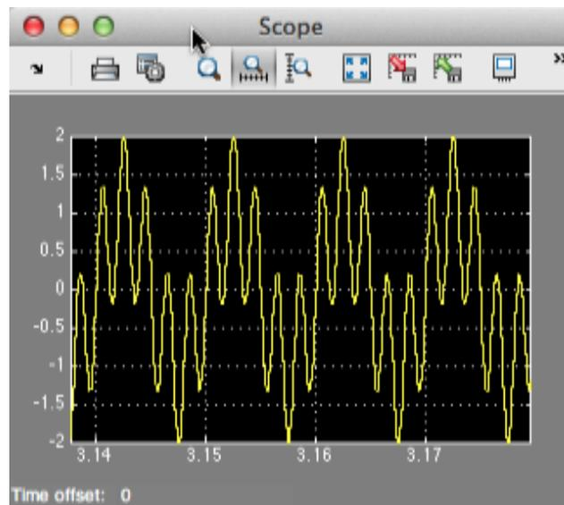
Figure 11. Scope Display of 100 and 500 Hz Sine Waves
