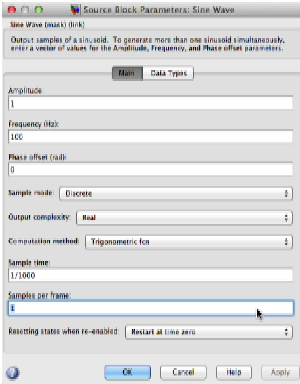
Figure 3. Sine Wave Source Block Parameter Window
