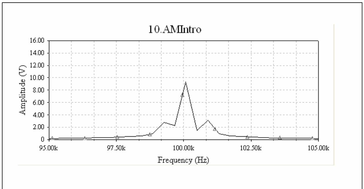
Figure 10-2 Frequency Spectrum of an AM Signal
