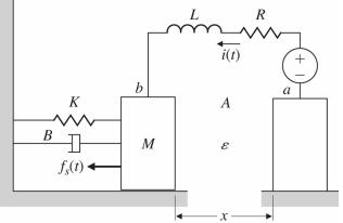
The system consists in part of a parallel plate capacitor connected into an electrical circuit. Capacitor plate a is rigidly fastened to the microphone frame. Sound waves pass through the mouthpiece and exert a force  $f_s(t)$  on plate b, which has mass M and is connected to the frame by a set of springs and dampers. The capacitance C is a function of the distance x between the plates, as follows:
