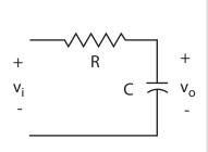
We have just developed the *transfer function* for the RC circuit. Now we will solve for  $v_o(t)$ .
