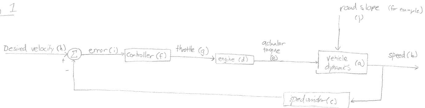
throttle: flow of fuel / air into engine
