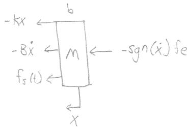
$\text{sgn}(\dot{x})$  returns the sign of  $\dot{x}$  (-1 or 1).  $fe$  is the electrical resisting force
