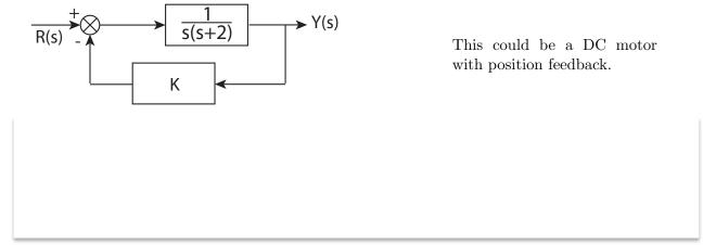
The response to a change in reference input is stable instead of continuing to integrate as in open loop. (Compare to example in Lecture 5.)
