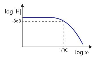
A sinusoid at frequency  $\omega_c = \frac{1}{RC}$  has been shifted in phase by 45° and reduced in magnitude to  $\frac{\sqrt{2}}{2}$  relative to the input.
