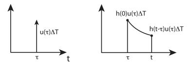
At any time t, the output y us a result of all past impulses, so:
