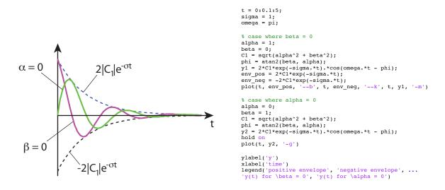
Real poles give a stable response when they are negative. Complex poles give a stable response when they have negative real parts.
