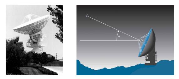
The antenna and drive parts have a moment of inertia J and a damping B; these arise to some extent from bearing an aerodynamic friction, but mostly from the back emf of the DC drive motor. The equation of motion is
