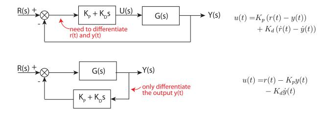
If the reference signal is noisy, it may be preferable to have the controller in the feedback path to avoid differentiating it. The feedback path is also better if the reference input makes step changes. (What will the input u(t) try to do in such cases?).
