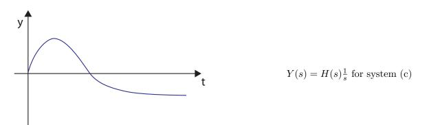
This characteristic can be seen in many real systems, including an inverted pendulum on a cart and highly maneuverable jet aircraft. We'll return to this later when we study frequency-domain analysis (Bode plots in particular) and can look at phase plots.
