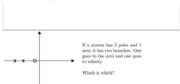
**<u>Rule 2</u>** Points on the real axis to the left of an odd number of poles and zeros are on the locus
