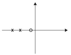
If a system has 2 poles and 1 zero, it has two branches. One goes to the zero and one goes to infinity.
