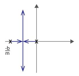
As K is increased, the open loop poles move toward one another before breaking away from the real axis and moving toward infinity.
