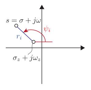
For any point  $s = \sigma + j\omega$ ,  $s - z_i$  is also a complex number.
