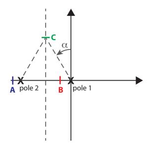
A:  $\phi_1 = 180^\circ$  (line goes from pole to test point)  $\phi_2 = 180^\circ$
