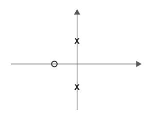
What does this system do? We know the real axis to the left of the zero lies on the root locus, but how do the poles get to the real axis?
