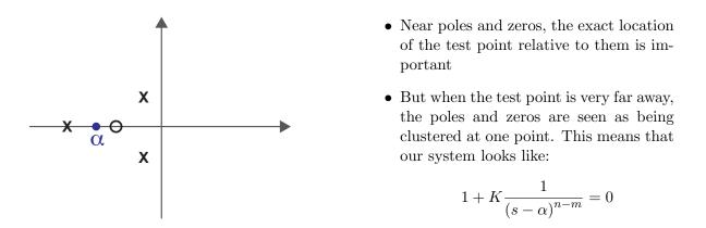
As test points are taken farther and farther away, it is only the net number of poles that becomes important. All of these can be treated as being at the single point  $\alpha$ .
