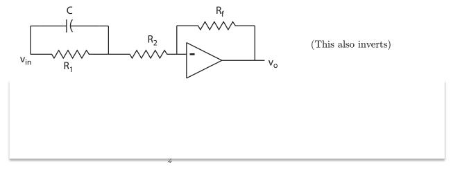
Analog implementation has the advantage of simplicity and speed (bandwidth). However, the controller characteristics are tied to these specific component values.
