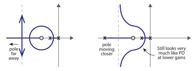
Lead compensators can be used to specify the location of the dominant pair of closed loop poles in order to meet performance specifications like rise time and overshoot. How do we build a lead compensator? One implementation is in the form of an analog circuit.
