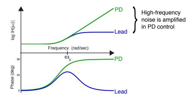
This gives a clearer explanation of lead compensation as a combination of PD control and a lowpass filter. This is literally true. The lead compensator does not amplify high-frequency signals as much as the PD controller. By changing the value of  $\alpha$ , we can make the lead compensator match the response (and behavior) of the PD controller over a certain frequency range.
