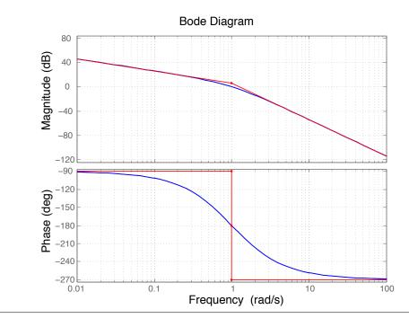
So what does this tell us about stability? When the points on the root locus become neutrally stable, they are purely oscillatory, so  $s = j\omega$ . We also know that since this "crossing point" is on the root locus, it must satisfy |KG(s)| = 1, and  $\angle G(s) = 180^{\circ}$ .
