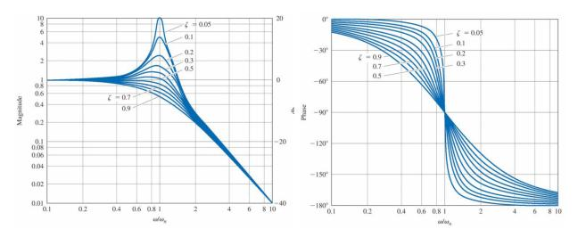
To sketch, the plot is centered around  $\omega_n$ , with a resonance peak and phase angle slope that are determined by the damping ratio.
