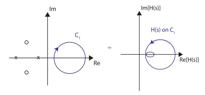
This can be done point by point for each test point on the contour  $C_1$ . The plot on the right is known in controls as a Nyquist plot. You can think of it as the real and imaginary components of H(s) (corresponding the vertical and horizontal axes), or as a polar plot of angles  $\angle H(s)$  and magnitudes |H(s)|, evaluated as s moves around a clockwise contour.
