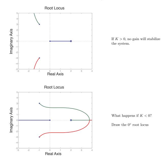
Note that the right half plane zero still means that poles move into the right half plane as  $K \to \infty$ . The negative gain doesn't change that, but may buy a period of stability.
