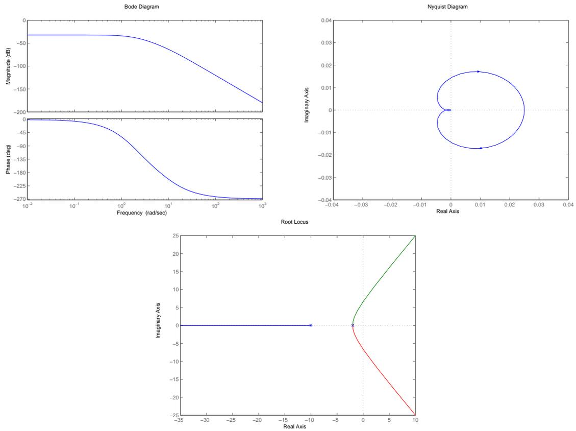
There are no open loop RHP poles, so we want no encirclements of  $-1$ . When the phase is  $-180^\circ$ , the magnitude is about 0.0017, so the gain would have to be around  $K = 1/0.0017 \approx 576$  for any encirclements of  $-1$ .
