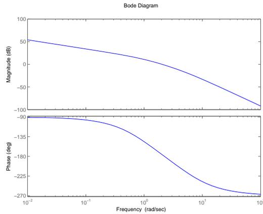
When the magnitude is about unity, the phase is around  $-180$ , so the phase margin is virtually non-existent. We know a lead compensator has phase up to  $90^\circ$  in the center, so we can put the lead compensator near the crossover frequency to boost the phase margin up to  $90^\circ$ . So a possible controller is
