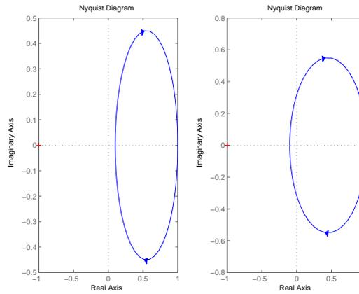
A RHP zero does not affect the number of encirclements required for stability. In particular, for these plants, we need 0 encirclements of  $-1$  for stability. (Of course, the Nyquist plots may be different for these two plants, so this condition may be met for different values of the gain  $K$ .)
