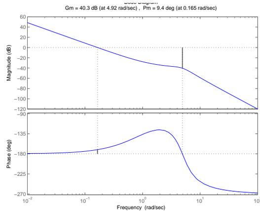
Note that we can use the Bode plot to tell stability; the magnitude crosses 1 only once, and increasing gain leads to instability (the asymptotics for the root locus will be  $\pm 60^\circ, 180^\circ$ ).
