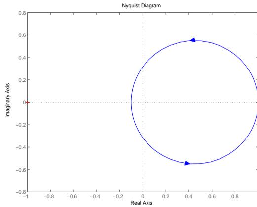
Unlike the first two plants, this plant has a RHP pole, so we require 1 encirclement of  $-1$  for stability. Therefore, the first plant will not be unstable for any  $K$ . The second plant will be unstable for  $K \geq 10$ , and the third plant will be unstable for  $K \geq 10$ .
