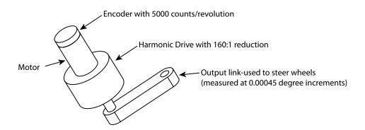
With this sampling rate and sensor resolution, we can easily use the continuous system techniques of this class to analyze the system. Furthermore, we can approximately obtain a PD controller by differencing the position output.
