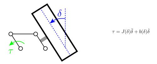
By paying attention to the linkage design (close to a parallelogram), we have made  $J(\delta)$  and  $b(\delta)$  roughly constant, so a reasonable model is:
