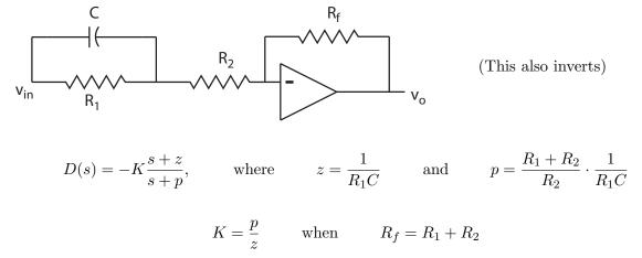
Analog implementation has the advantage of simplicity and speed (bandwidth). However, the controller characteristics are tied to these specific component values.
