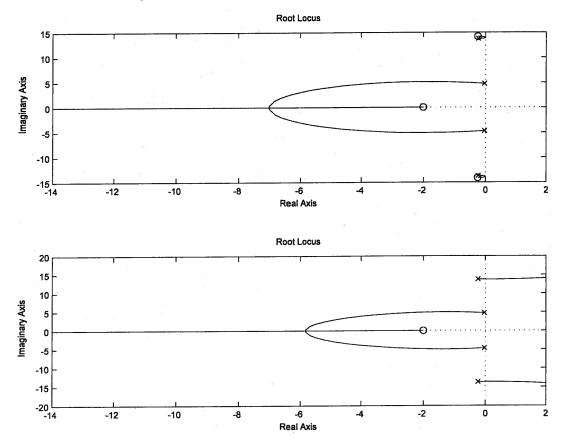
We can intentionally add zeros near lightly damped poles to get the same effect. This is notch compensation:
