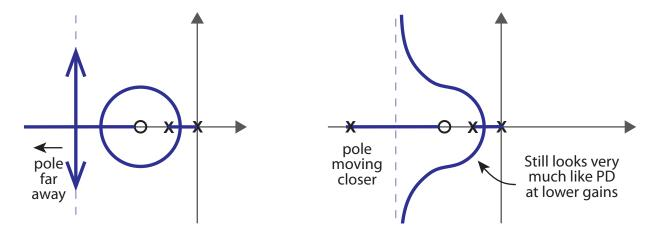
Lead compensators can be used to specify the location of the dominant pair of closed loop poles in order to meet performance specifications like rise time and overshoot. How do we build a lead compensator? One implementation is in the form of an analog circuit.
