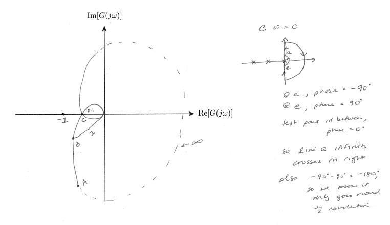
b. (10 pts.) Imagine that G(s) is placed in a feedback system whose characteristic equation is 1 + KG(s). As K varies from 0 to infinity, describe the number of closed-loop right-half-plane poles and say whether the system is stable or unstable. Also, give the value(s) of K at which any transition in stability takes place. (Hint: You can return to the Bode plot to help with this.)
