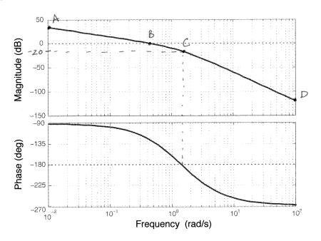
a. (5 pts.) Sketch the Nyquist plot for G(s). Identify at least 4 important points (A, B, C, and D) on the Bode plot and show their corresponding positions as accurately as possible on the Nyquist plot. Include the -1 point on your Nyquist plot. Show any calculations needed to explain the behavior of any infinite points Nyquist plot. Draw arrows corresponding to the direction of the contour, and use a dashed line to indicate the parts of the plot at infinity.
