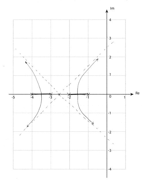
b. (9 pts.) Calculate the following guidelines for sketching the root locus  $1 + K_pG(s)$ , and draw asymptotes on the s-plane in part a.
