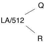
Block to be accessed = Q + starting address Displacement into block = R
