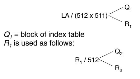
$Q_2$  = displacement into block of index table  $R_2$  displacement into block of file:
