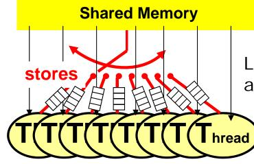
Loads(each thread can have at most one outstanding load)
