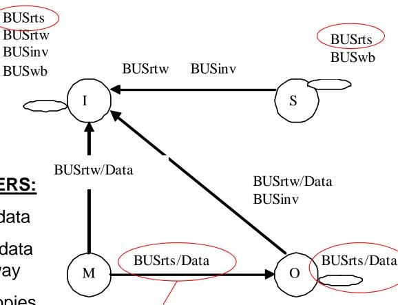
Input-signal/Reply-signal Meaning: If you are in state M and see BUSrts, goto state O and reply with Data
