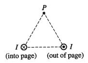
56. Current I flows into and out of the page in two parallel, long, straight wires that are fixed at two vertices of an equilateral triangle, as shown above. The net magnetic field at the third vertex (point P) due to these currents is in which of the following directions?
