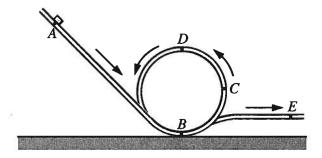
A block released from rest at position A slides with negligible friction down an inclined track, around a vertical loop, and then along a horizontal portion of the track, as shown above. The block never leaves the track.
