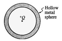
Charge +Q is located at the center of the hollow metal sphere shown in cross section above. The net charge on the sphere is zero.
