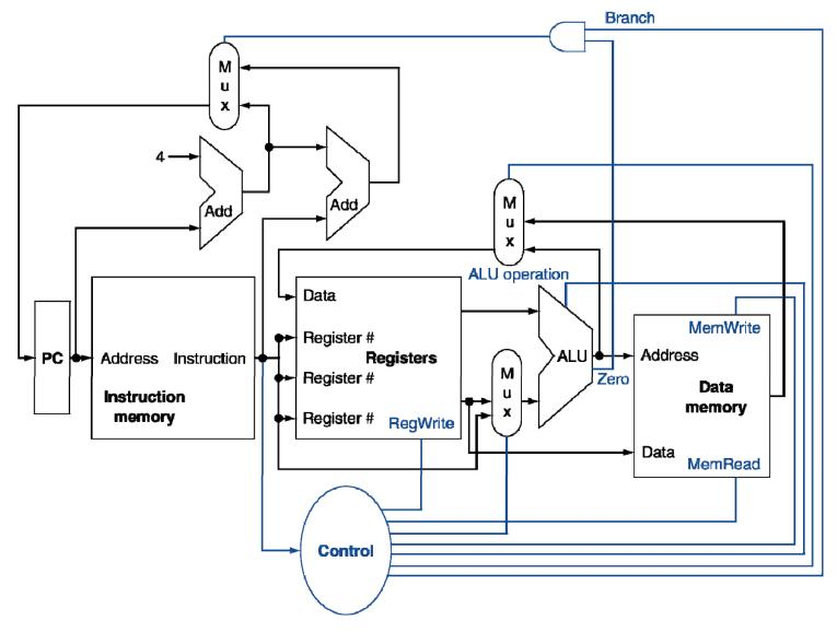
**Problem:** Consider the instruction: AND Rd, Rt, Rs. What are the control signals generated by the control unit in this figure?
