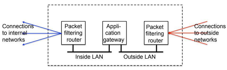
Adapted from Fig. 9-28 in "Distributed Systems", by Tanenbaum and Van Steen
