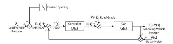
The error, e(t) or E(s), is extremely important. If this value gets too large, the cars may collide. We therefore want to look not only at the transfer function from reference to output, but also at the transfer function from reference to error:
