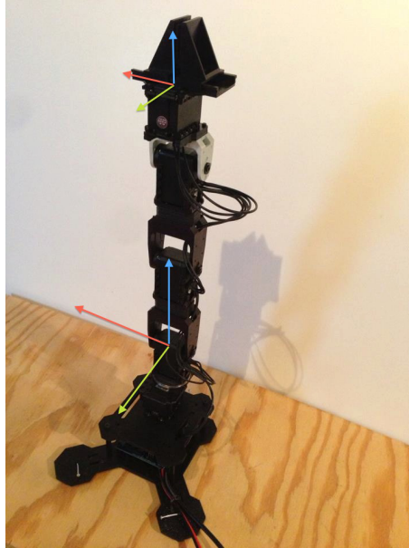
Figure 10.1: Pincher robot at rest, with all joint angles at 0. The chosen base frame S and tool frame T are shown as RGB coordinate frames.
