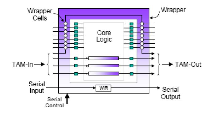
• Core internal scan path & Wrapper Cell Register are connected in parallel to TAM by a Core Test instruction
