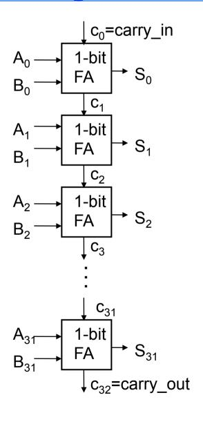
■ Just connect the carry-out of the least significant bit FA to the carry-in of the next least significant bit and connect . . .
