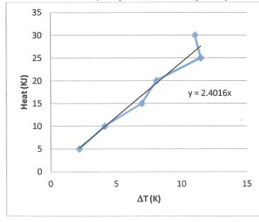
From the colibration of the Colorimeter we con coloriste the Ear as the stope of 9 vs DT. BAL = 2.40 KJ
