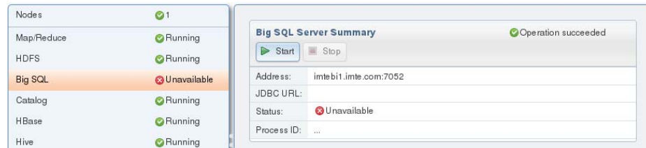
Figure 9 – Web Console showing Big SQL service stopped
