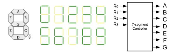
7. Implement the 7-segment using a 4-selector DEMUX and Or gates.
