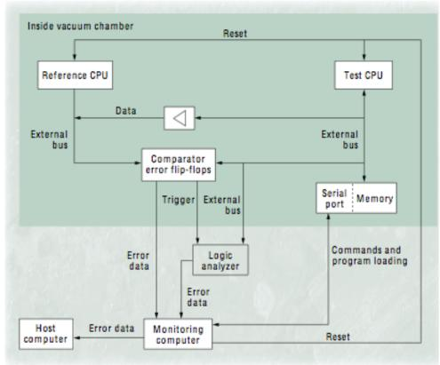
**FIST from Chalmers [Karlson'1995]**: Used a Vaccum chamber in which an ionizing source was placed. A second non-faulty processor was used for state comparision.
