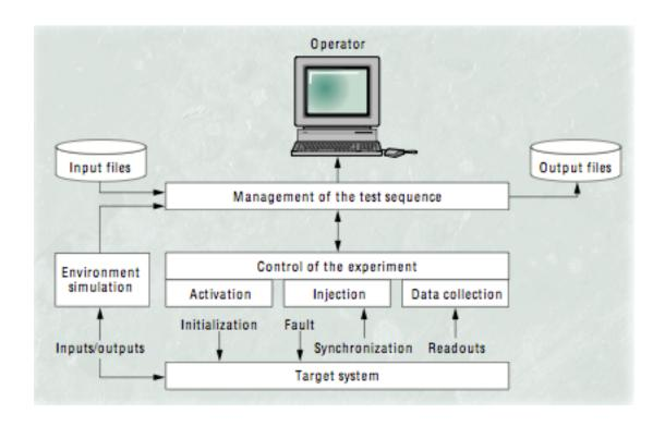
Messaline from CNRS [Arlat'1990]: Can perform probe-based and socket-based injection. used for evaluating safety-critical systems such as railway control system
