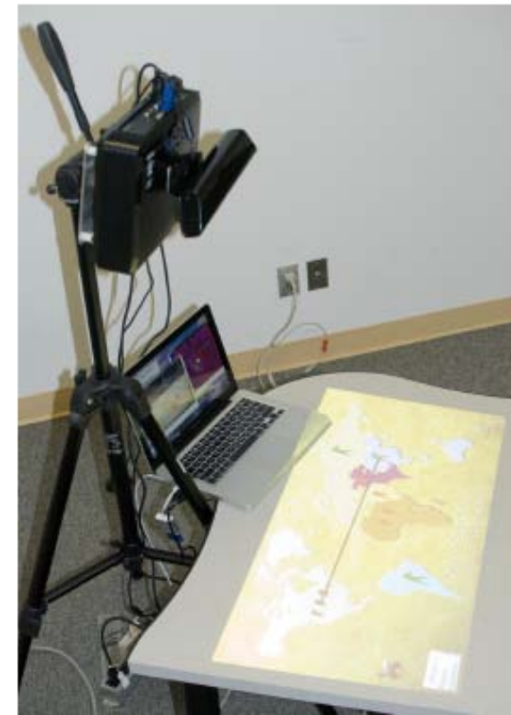
Figure 1: Interactive Spaces configuration. The mobile system is composed of Kinect attached to the top a short-throw projector and is mounted on a tripod to ease portability and installation.
