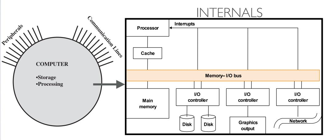
Bus = control lines + data lines Control lines carry requests, acknowledgements, type of information Data lines carry data, complex commands, or addresses
