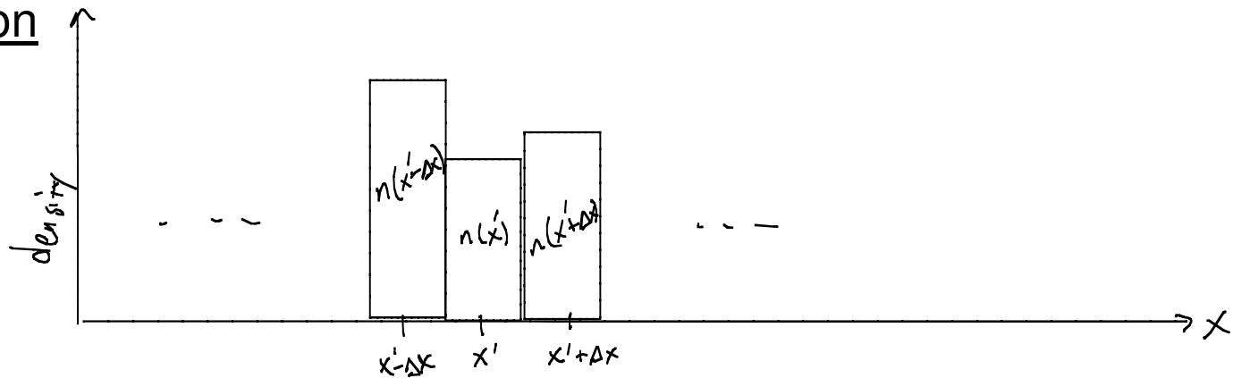
Rate equation: During every element of time  $\Delta t$ , half the particles within range  $\Delta x$  will go left and half go right. The number/density rate of change at  $x=x'$  is
