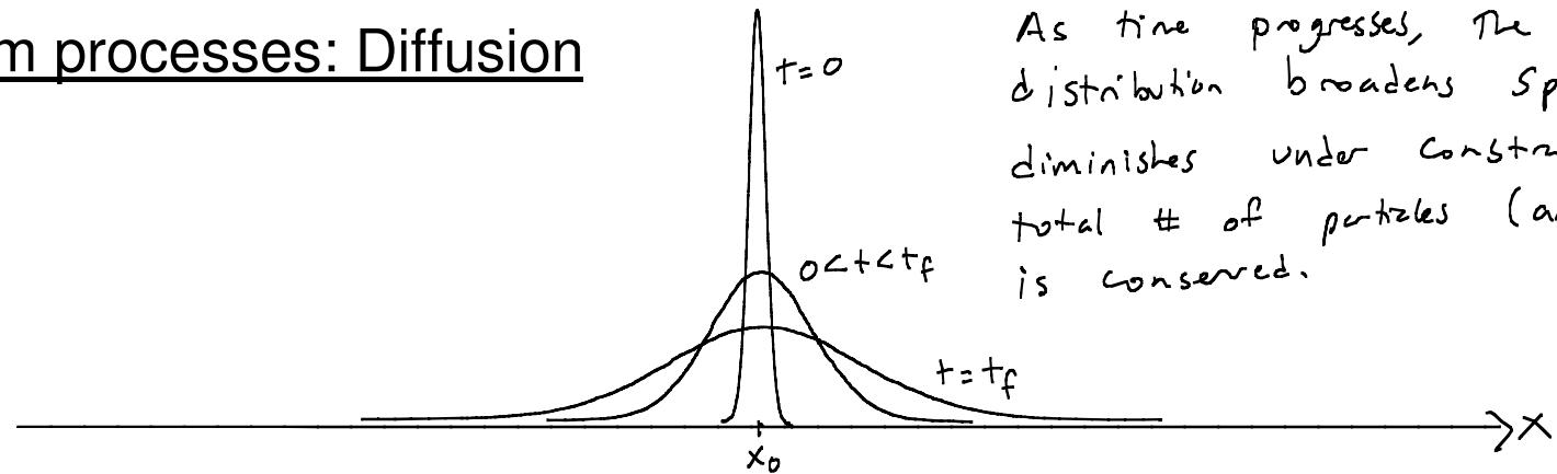
We can simulate this process by following the "random walk" of a large number of particles that start @  $x=x_0$  and move left or right at every timestep until  $t=t_f$ .
