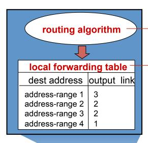
routing algorithm determines end-end-path through network
