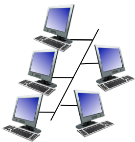
shared wire (e.g., cabled Ethernet)
