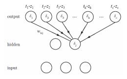
(Duda et al. Pattern Classification 2000) The sensitivity at a hidden unit is proportional to the weighted sum of the sensitivities at the output units:
