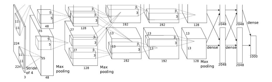
Figure1. ImageNet CNN Model
